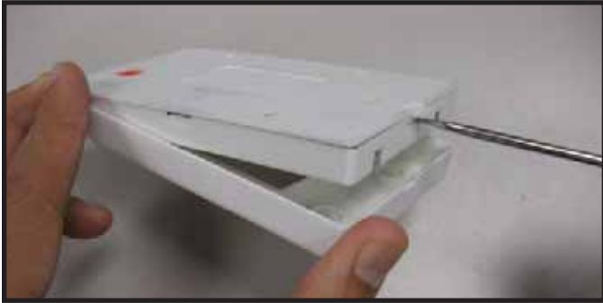
Figure 1. Wall Switch Disassembly
